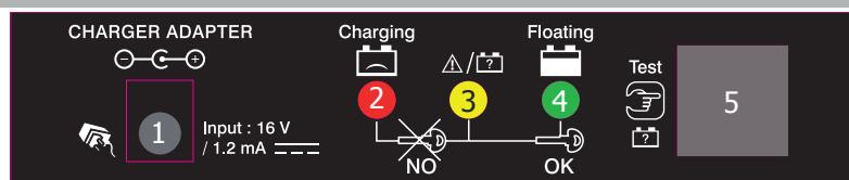
**1** Connection for the charger-adapter. Use only the charger-adapter provided with the product.
